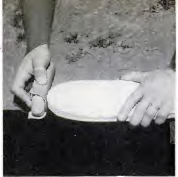
After cutting the rounded front end of the skis, carefully sandpaper away all roughness and sharp edges
